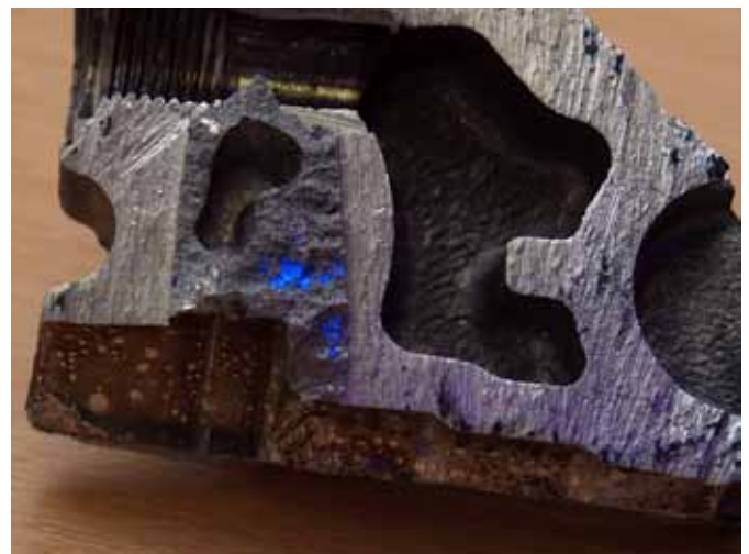
Figure 4: Section of Casting Impregnated with Sealant (Under UV Light)
